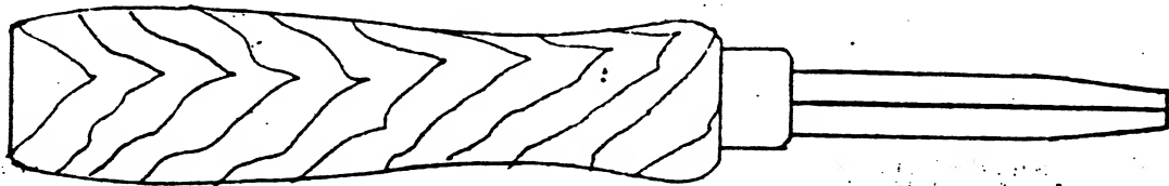
3-CORNERED FILE TOOL, SPECIAL GRIND, FOR REMOVING BROKEN OR STUCK SECTIONS
